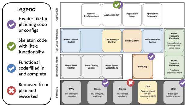
The clocks file is removed since configurations will be done for their own MCU or board specific functions. New files for current sensing will be required at the second lowest layer. And ADC firmware file will likely need to be added. The DMA will probably be a configuration thing only so there probably won't be a separate file for that.
